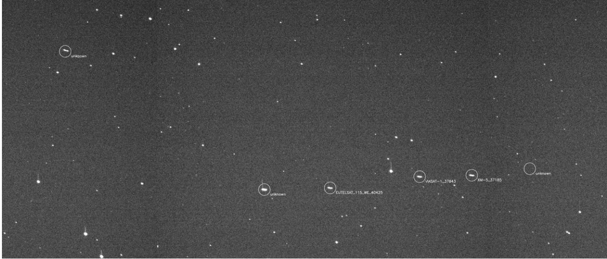
Fig. 5 identification result of GEO object in sample combined image. IGSO like object detected (left-up)
