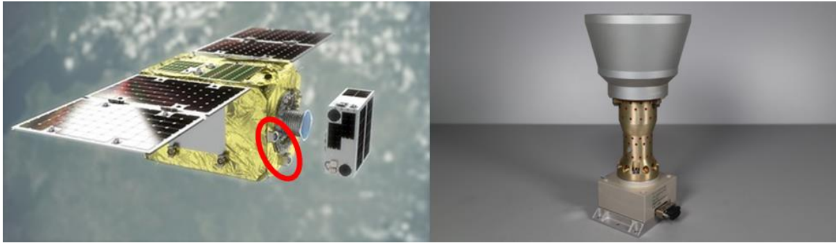
Fig. 2. Left: ELSA-d servicer and client spacecraft with the long-range and short-range cameras circled in red. Right: The Malin Space Science Systems ECAM-C50/M50 which is used as an example in this study [6].
