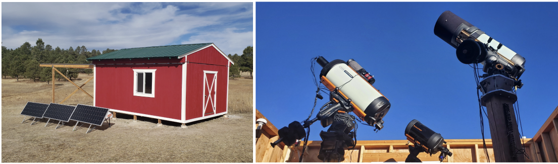
Fig. 1: Pine Park Observatory is a roll off shed design housing three telescopes. The telescope furthest to the right is the 8" Celestron used for the experimentation reported in this paper.
