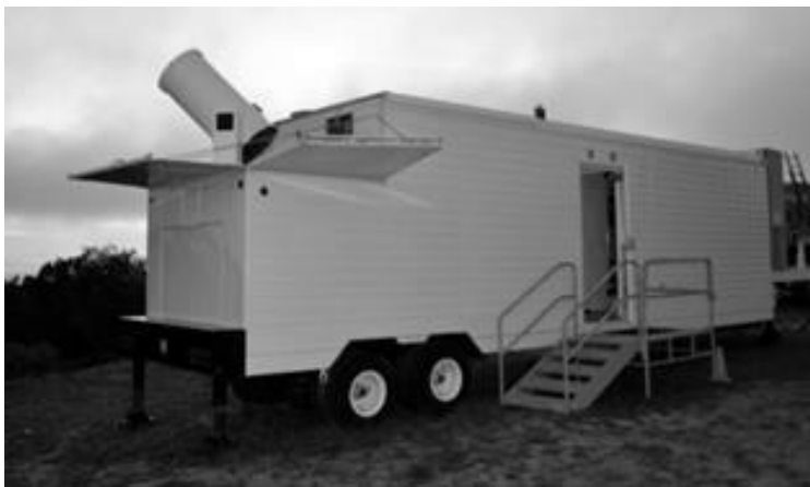
Figure 1: The Satellite Tracking and Illumination LADAR Trailer, showing the roll-back roof and the 0.5 meter Coudé path telescope. The telescope sits on a 5'x12' optical bench inside the trailer.
