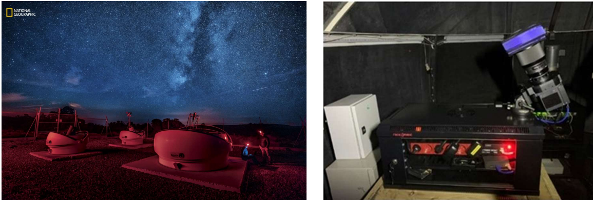
Fig. 3. Deimos Sky Survey dome (left) and the control system setup with 85mm lens (right).
