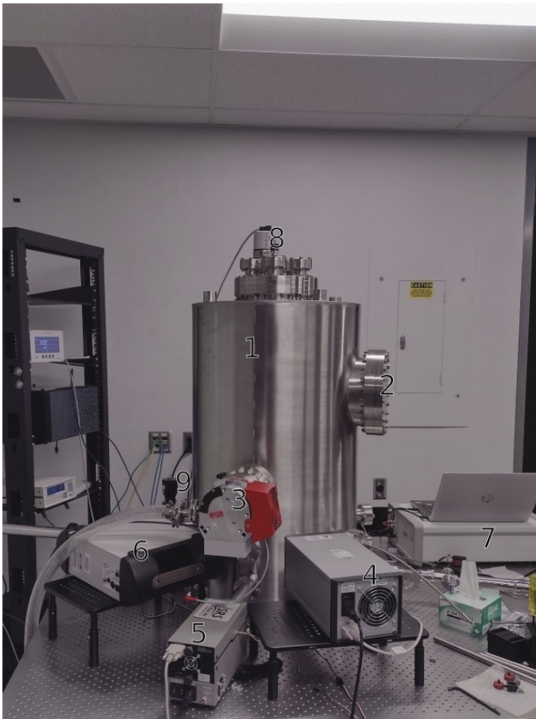
Fig 4: The side view of the phase angle vacuum chamber, with numbers labeling major components. 1. is the main chamber, 2. is a 10in. Access port. 3. is the ultrahigh vacuum Pump, 4. is the combined visible and deuterium lamp. 5. is the residual gas analyzer, 6. is the Vis-NIR spectrometer, 7. is the FTIR, 8. is the vacuum gauge, 9. is the gate valve for sample entry.
