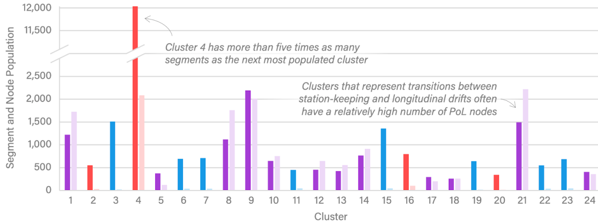
Fig. 3: Segment and PoL node population of each cluster. Segment populations are shown in dark colors; PoL node populations are shown in light colors. The number of PoL nodes relative to the segment population of a cluster can be used to sort the clusters into the three broad behavioral classes: station-keeping, shown in blue; longitudinal shift, shown in red; and transitioning between the two, shown in purple.
