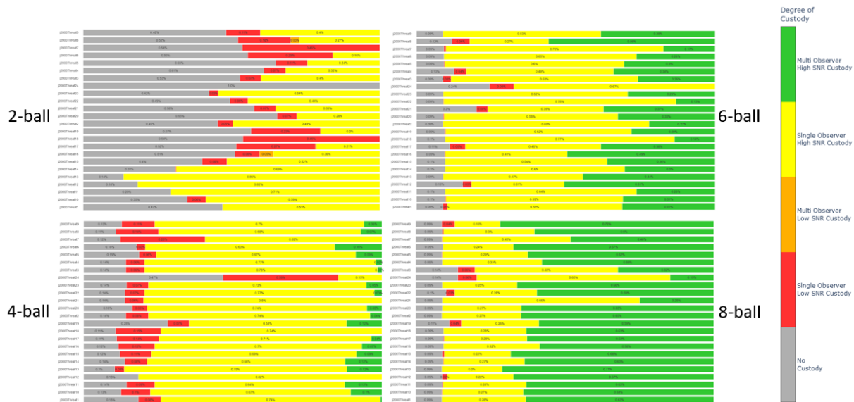
Fig. 12: Plot of the effect of evenly-spaced patrol sat assets along the GEO belt. Upper left: 2 assets at 180^\circ separation. Lower left: 4 assets at 90^\circ separation. Upper right: 6 assets at 60^\circ separation. Lower right: 8 assets at 45^\circ separation.
