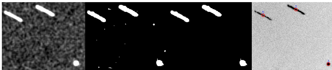
Fig 3.2. From left: image prior to object extraction, pixels above threshold value, selected pixel groups after filtering, raw image with centroid positions (red circles) of selected pixel groups overplotted.
