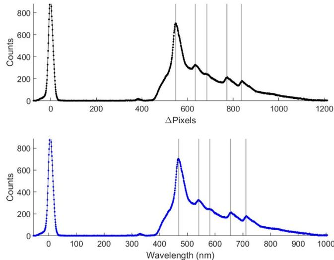
Fig. 8. The spectrum of HIP33165 in pixel space (top plot) and wavelength space (bottom plot) for the 200 lines/mm diffraction grating on the USAFA-1m telescope.
