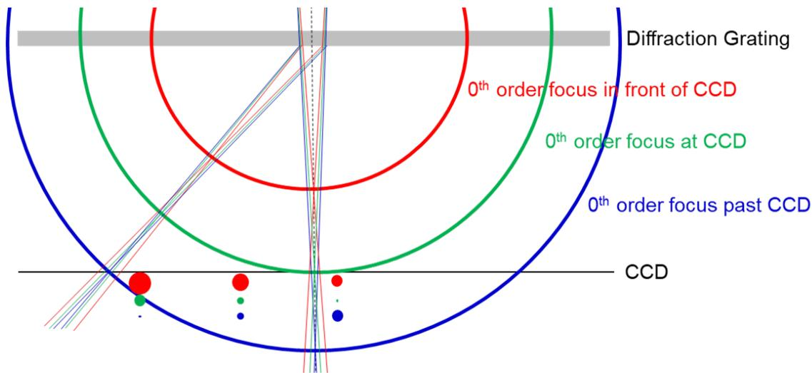
Fig. 5. First-order focusing issue for large-format CCDs when zero-order is in focus (blue), the first-order is more and more out of focus the further from the zero-order it is. By focusing the zero-order past best focus (orange), more of the first-order can be put into focus.
