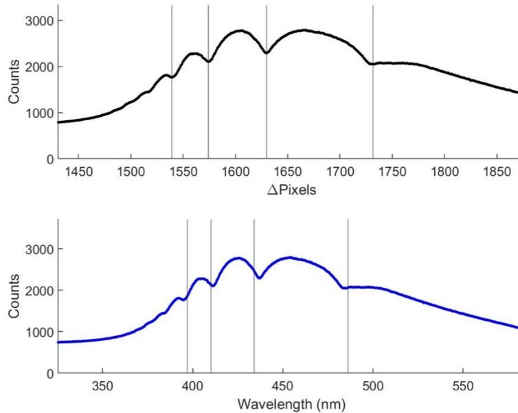
Fig. 11. Pixel-to-wavelength calibration using Castor’s spectrum resulting in a slope of  $0.47 \pm 0.02$  nm/pixel and offset =  $-324 \pm 34$  nm. The Hydrogen Balmer absorption lines are located at 397 nm, 410.2 nm, 434 nm, and 486.1 nm.
