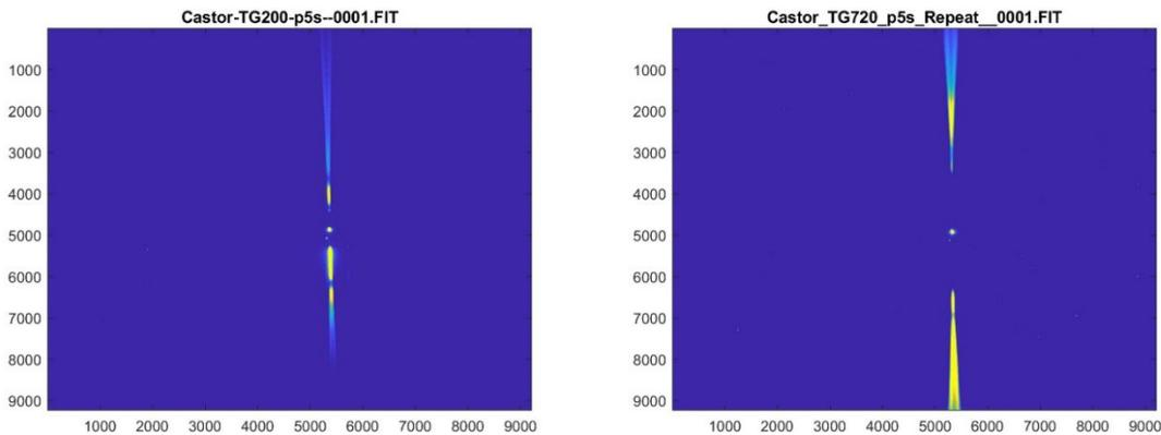
Fig. 3. USAFA-1m telescope 0.5-s exposures of Castor on 2023 Feb 25 using the 200 lines/mm grating (left) and 720 lines/mm grating (right).
