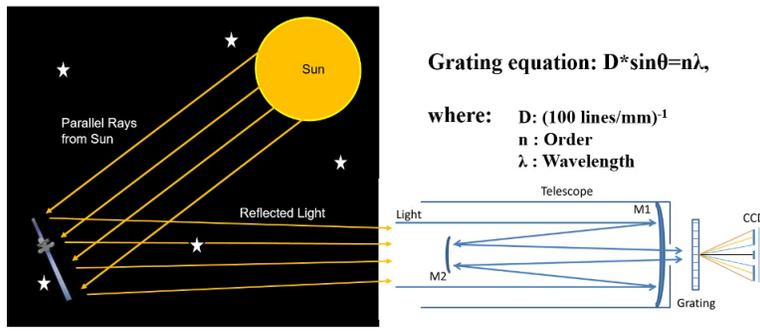
Fig. 2. Image shows the imaging scenario between the sun, the satellite, and the observer. Light reflects off the satellite, goes through the telescope where it passes through the diffraction grating. The light is then spread out onto the focal plane based on the grating equation.
