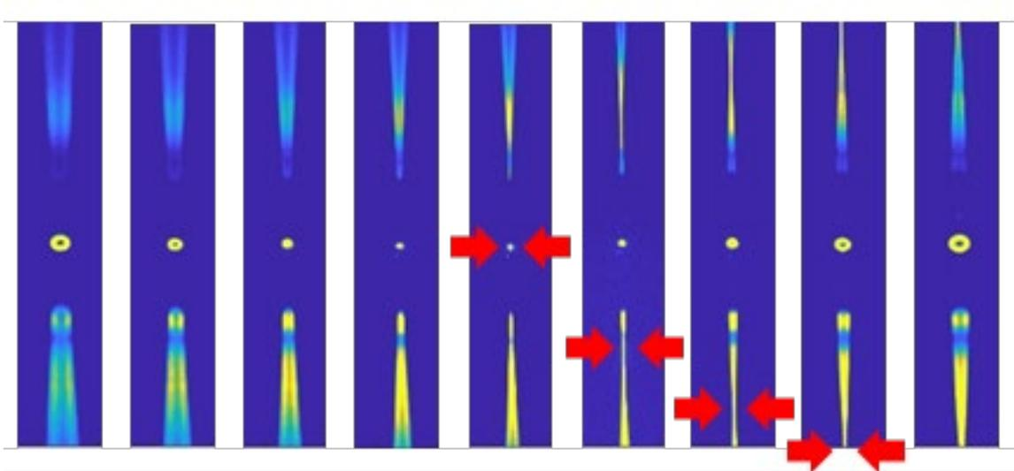
Fig. 4. Images of zero and higher orders of Castor using USAFA 1-m telescope and 720 lines/mm grating (2023 Feb 25). The center image shows the zero-order in focus, while the images left and right of the center image shows how the higher orders are affected when we defocus in either direction. The lefthand images are when the zero-order is inside the focal length while the righthand images correspond to when the zero-order is outside the focal length.
