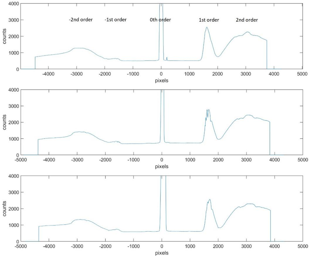
Fig. 6. Extracted spectra for Castor images (0.5-s exposures) at three different focuses. Zero-order in focus (top), between first and second orders in focus (middle), end of second order in focus (bottom).
