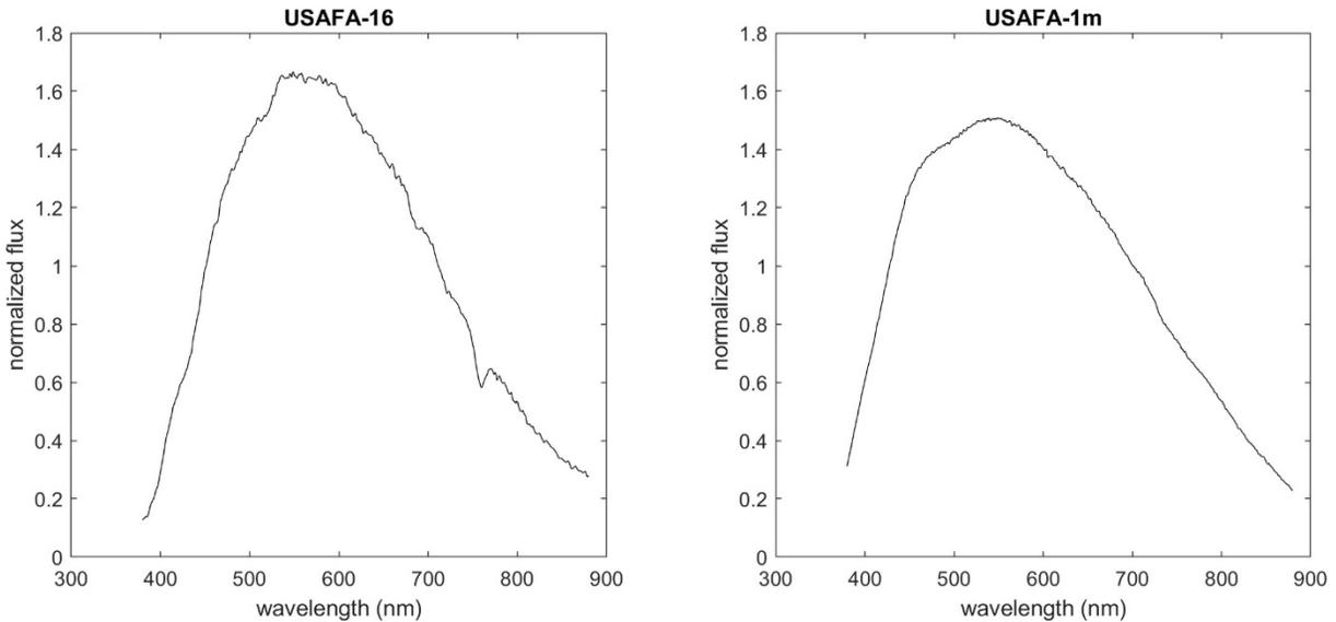
Fig. 9. HIP51993 (G2V type star) spectra using the 100 lines/mm diffraction grating with the USAFA-16 telescope (left) and the 200 lines/mm diffraction grating with the USAFA-1m telescope (right).
