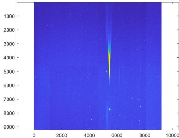
Fig. 10. HIP33165 (zero-order near center of image) using USAFA 1-m telescope and 720 lines/mm grating (2023 Feb 25). Higher orders are defocused the further from the zero-order, which is most evident for the brightest star also in CCD frame.
