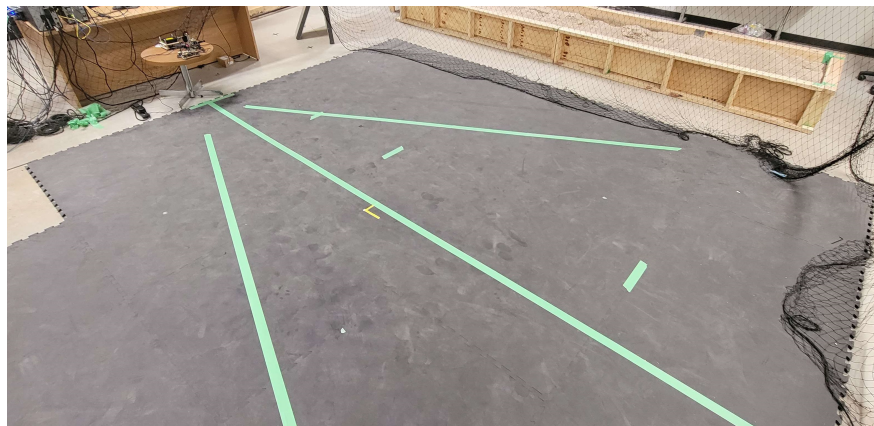
Fig. 10: Slow testing area, the Vicon system provides motion capture coverage throughout the entire OLTS FOV marked by tape.
