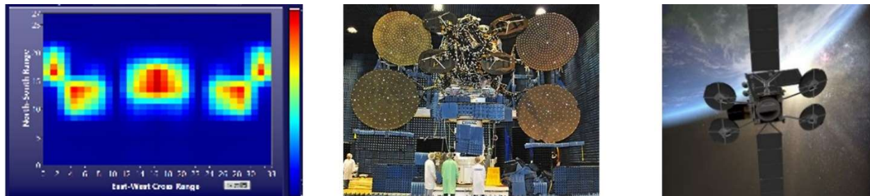
Fig. 11 Real ISAR images of VIASAT-1, March 2023 (ISAR image, left, antenna deployment testing, center, Artists impression of On-orbit Configuration, right).
