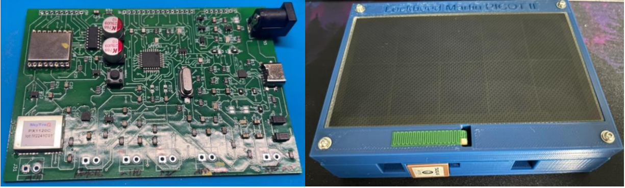
Fig. 11: Lockheed Martin's GPS Transponder Circuit Board (Left) and Prototype Transponder (Right)
