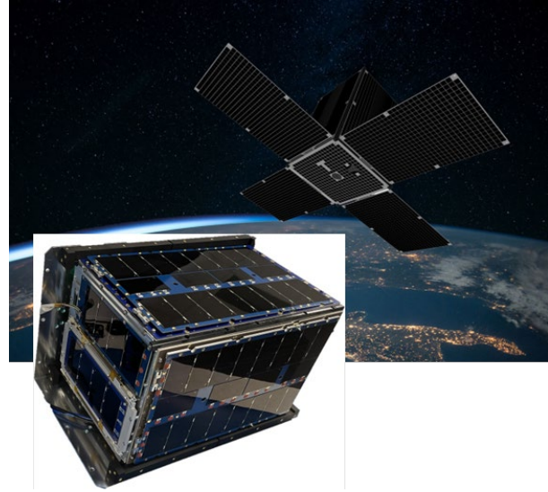
Fig. 5: Drawing of Inovor's Hyperion SDA sensor on 12U Apogee bus flying in LEO with the engineering design unit shown in the inset.
