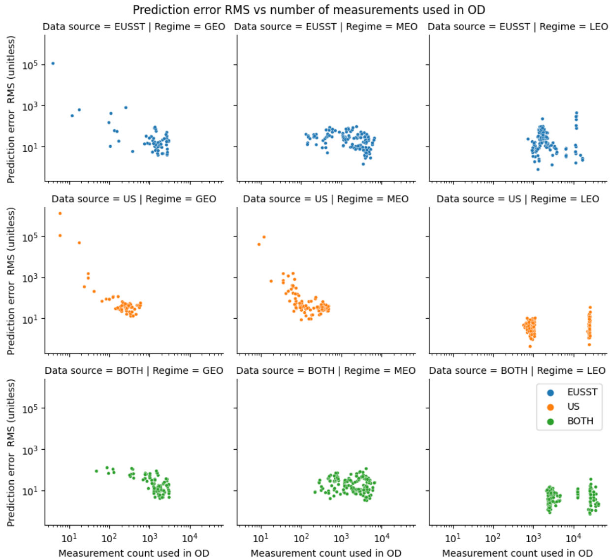
Fig. 8: Representation of prediction error vs. number of observations used in OD, both by regime and data provider
