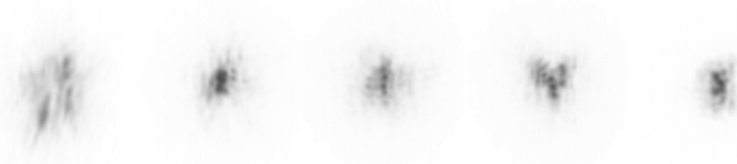
Fig. 2: Five example (simulated) broadband data frames ( 400 \text{ nm} \leq \lambda \leq 984 \text{ nm} .) for observations with a 3.6m aperture at an zenith angle of 0 degrees through turbulence with r_0 = 17 \text{ cm} at 500 nm. We use a negative color table to better highlight the speckle structure.
