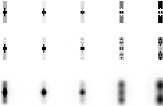
Fig. 3: Top row: The true intensity distributions at (left to right) 400 nm, 474 nm, 582 nm, 753 nm, and 984 nm. Middle row: The corresponding recovered intensity distributions from 80 data frames and 1,000 iterations. The zenith angle was 0 degrees, the telescope aperture was 360 cm, and r_0 = 17 cm. Bottom row: The corresponding intensity distributions for observations with diffraction-limited resolution.
