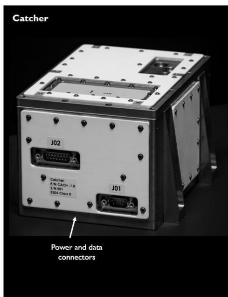
Fig. 7. Photograph and summary of the primary interface and host accommodations for the Catcher prototype.
