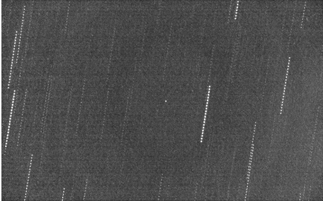
Fig. 1. GEO satellite RSO-tracking image (composite of 21 images on 2s centers) collected with the GEOStare2 CubeSat. The target satellite is the dot in the image center. The strings of dots are stars streaking across the sky.
