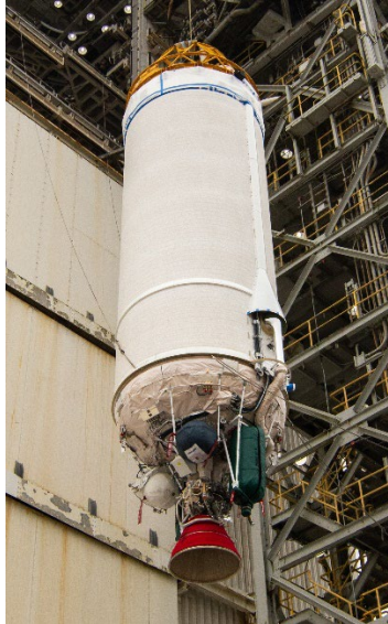
Figure 3 An Atlas V Centaur upper stage (single engine variant) [10]. The stage has a diameter of 3.05 m, and length of 12.68 m to include the nozzle, and an inert mass of 2,243 kg with the primary tank comprised of stainless steel 20 mils (~51 mm) thick.
