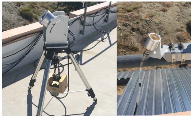
Fig. 3: Polaris image motion monitor and solar scintillometer at TMF. Polaris monitor is located on the roof of OCTL and at a height above RINGSS.
