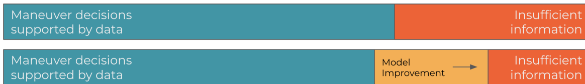
Fig. 3: Top – Categorization of conjunction events into those that support informed maneuver decisions with sufficiently small uncertainty (blue) and those that do not support the decision due to unacceptably large uncertainty at the MCP (orange). Bottom – The right-shift of well-supported decisions enabled by this approach (yellow overlapping the orange zone) with minimal wasted effort (yellow overlapping the blue zone). The yellow box illustrates the events impacted by the output of the model; it mostly overlaps the orange zone, which indicates the value lift in that those events have been positively affected with improved information, while the small overlap of the blue zone indicates that those events would have had sufficient information even without intervention.
