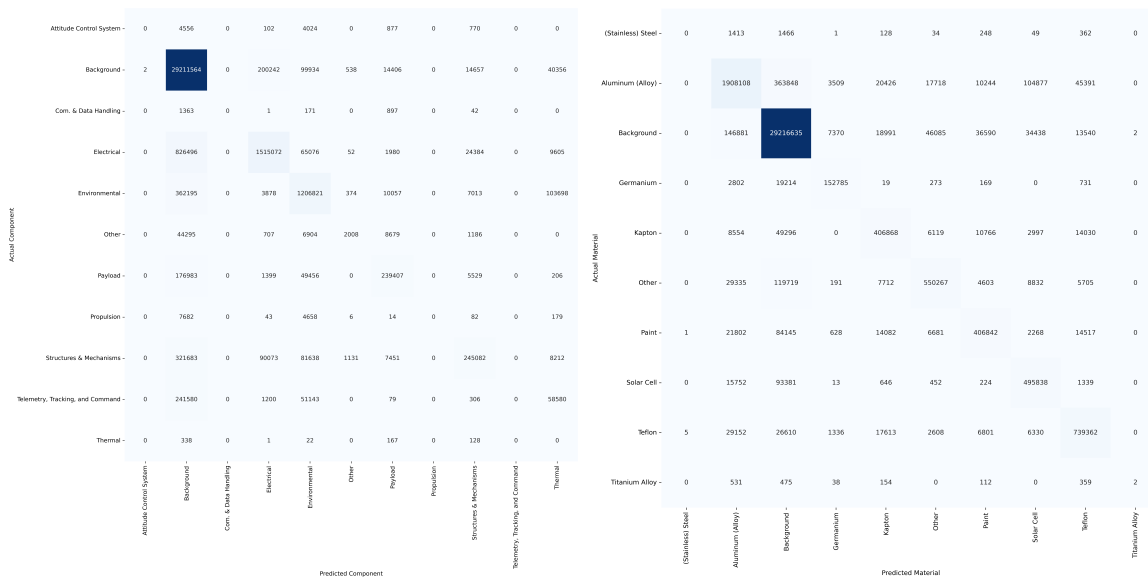
Fig. 8: These confusion matrices highlight the impact of class imbalance in our Hybrid Component (left) and Material (right) models, with a significant number of false positives for underrepresented classes like Propulsion and Titanium Alloy, while more common classes like Background, Electrical, and Aluminum Alloy dominate predictions.
