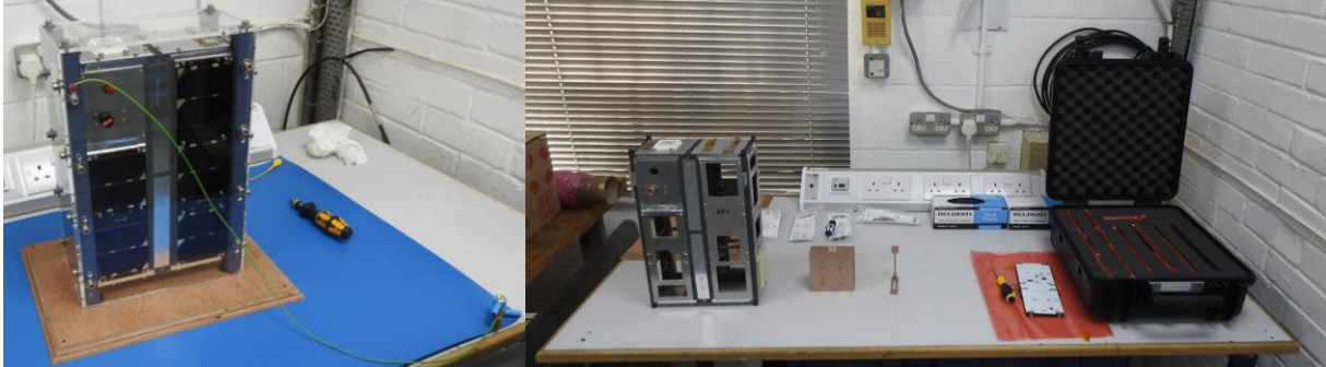
Fig. 4: Photographs showing the CubeSats in the measurement preparation room with the FM (left) in a protective case on an anti-static mat, and the EM set up (right) including the solar panel case, without these safety precautions.
