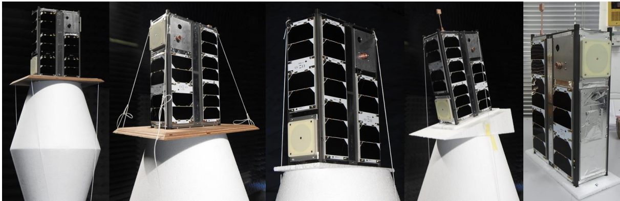
Fig. 8: Photographs showing the five CubeSat configurations measured. From Left to Right: FM, EM (FM set up), EM Magnetometer Stowed, EM Magnetometer Deployed (on 15^\circ Great Circle Cut wedge), EM Solar Panel replaced.
