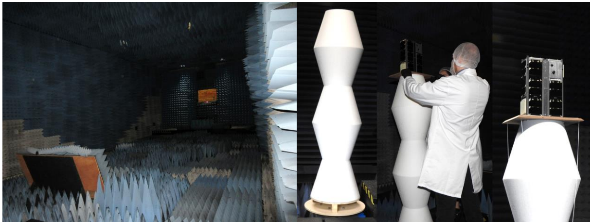
Fig. 5: Photographs showing the measurement chamber complete with RAM pyramids and antenna window at the end; the polystyrene column and the CubeSat team installing the FM onto the column.
