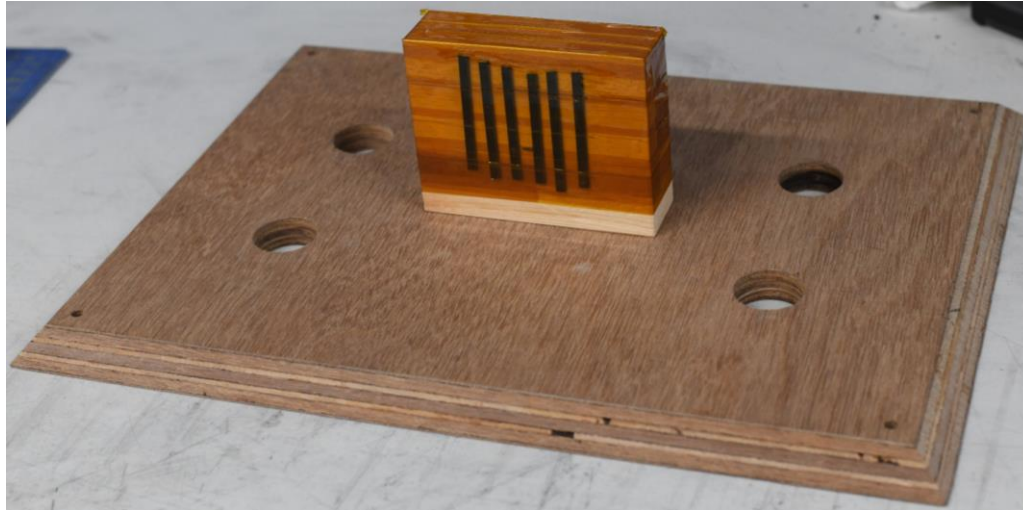
Fig. 3: Photograph of the wooden interface piece produced for safely securing the FM to the polystyrene column. Includes a vertical block that inserts into the FM and four holes for the corners of the FM to sit securely. Four small holes for affixing strings can also be seen in the corners of the interface.
