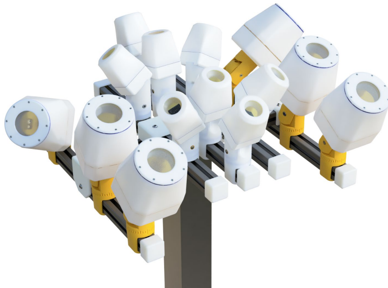
Fig. 2. A render of the Luciole camera system. Wide-field 8 mm cameras are in the middle while the narrow-field 25 mm cameras are at the edges of the battery.
