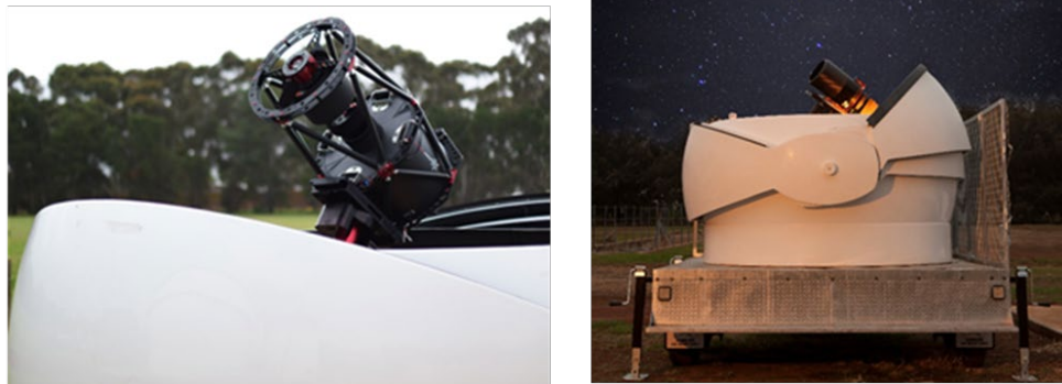
Figure 3. Fixed 50cm telescope (left) and the transportable 20cm telescope (right) of the DSTG optical observatory
