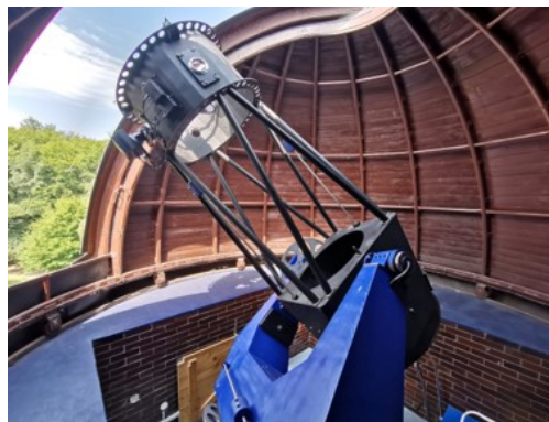
Fig. 1: The AGO70 newton telescope on fork equatorial mount. Credit: Stanislav Griguš
