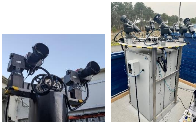
Fig. 4. “Classical” survey sensor and (left) and “Panoptès” survey sensor (right)
