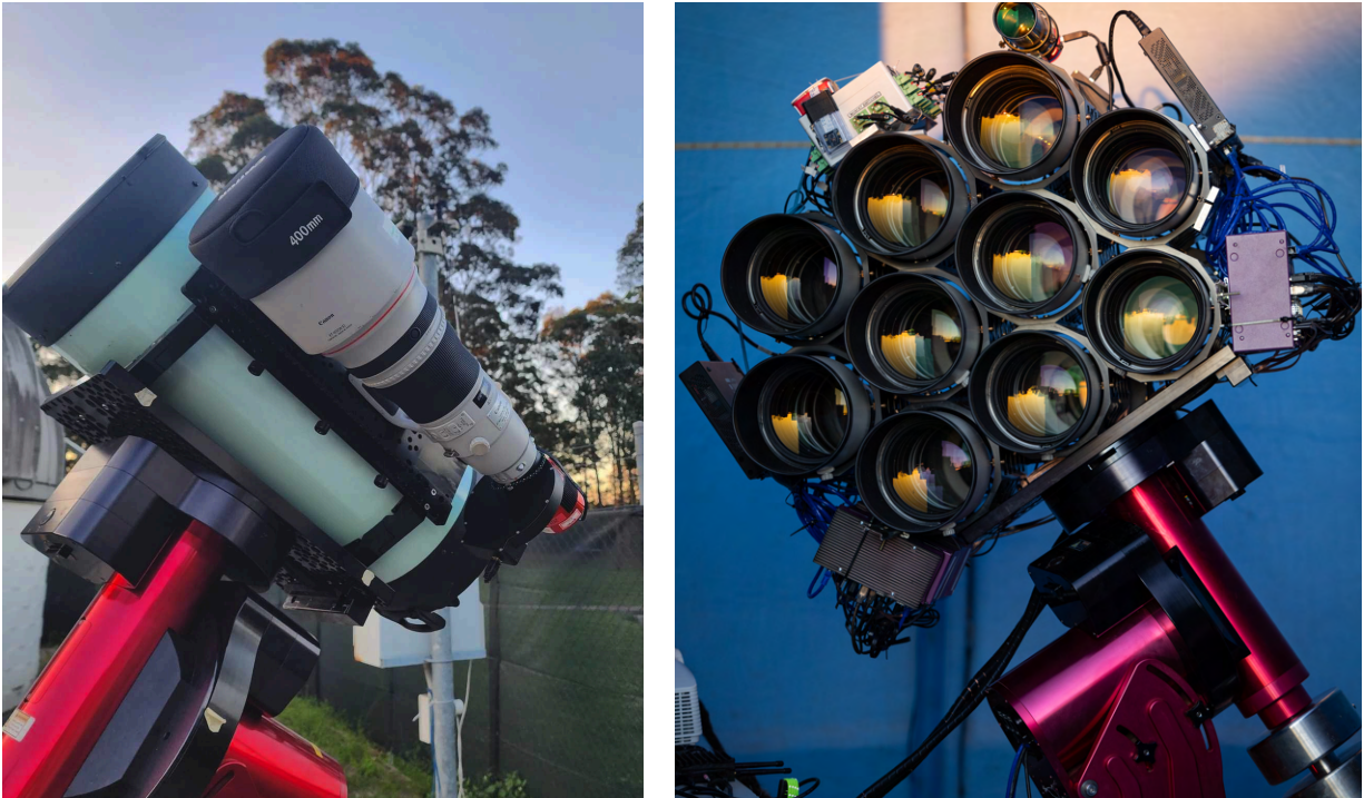
Fig. 1: Left, The Huntsman Telescope Pathfinder consisting of a single Canon lens used in this work. The Rowe-Ackermann Schmidt Astrograph our setup is attached to is not used in this work. The unit is located at Macquarie University Observatory, Sydney, Australia. Right, The Huntsman Telescope facility located at Siding Spring Observatory, Australia. Both telescopes use Canon 400 mm f/2.8 lenses with a pixel scale of 1.24'. The 10 lenses are configured to cover the same field of view of 1.89^\circ \times 1.26^\circ .
