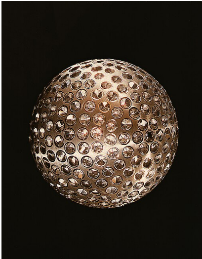
Fig. 1: LAGEOS-1 satellite (ILRS) designed to provide an on-orbit laser ranging target (NASA/Marshall, Public domain, via Wikimedia Commons)
