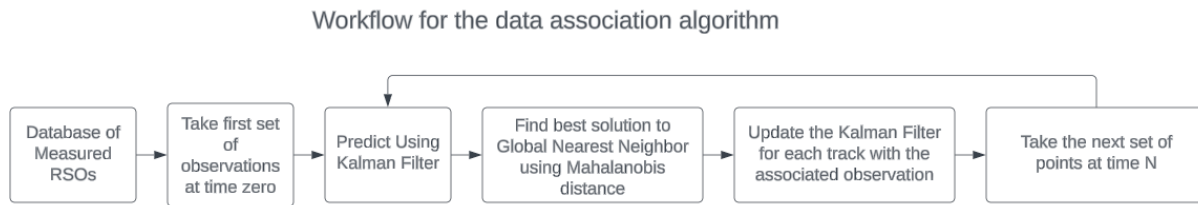
Fig. 10: Illustrates how the data association algorithm joins consecutive observations together, taking observations and forming a track.
