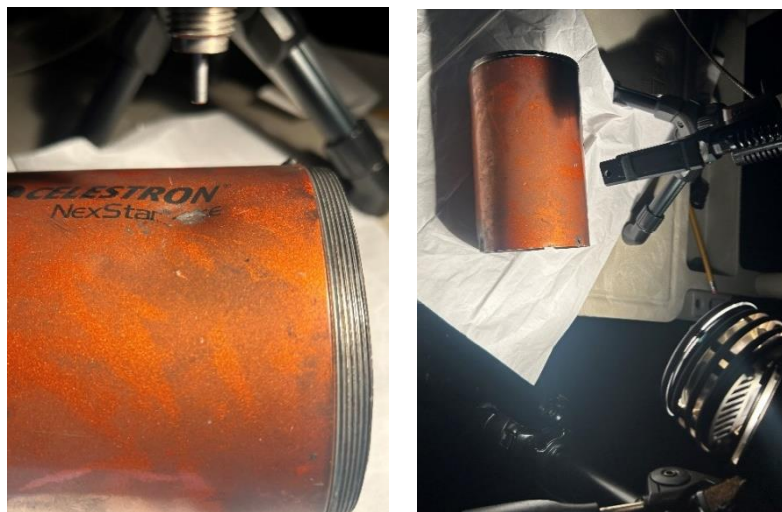
Figure 10. Digital images of the recovered DebrisSat telescope housing
