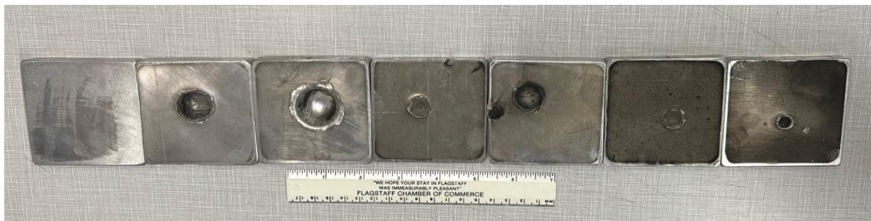
Figure 5. Al plates used for alignment tests in a two-stage light-gas gun. All targets were impacted \sim 5.5 km/s, at a chamber pressure of \sim 40 mtorr. From left to right, projectiles used in each test were as follows: pre-test blank, Lexan cylinder (no sabot), Lexan cylinder (no sabot), Al sphere, Lexan cylinder (no sabot, projectile partially impacted sabot catcher), Al sphere, stainless steel sphere.
