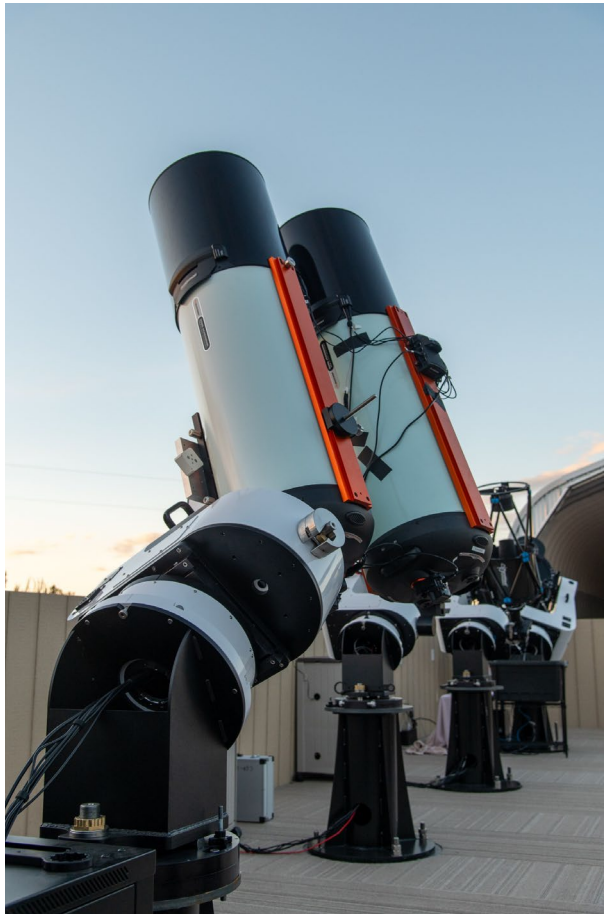
Figure 4. The AURORAS testbed system features dual Celestron RASA 36 cm telescopes equipped with an event-based camera and a CMOS sensor to enable simultaneous side-by-side observations with both sensor types.
