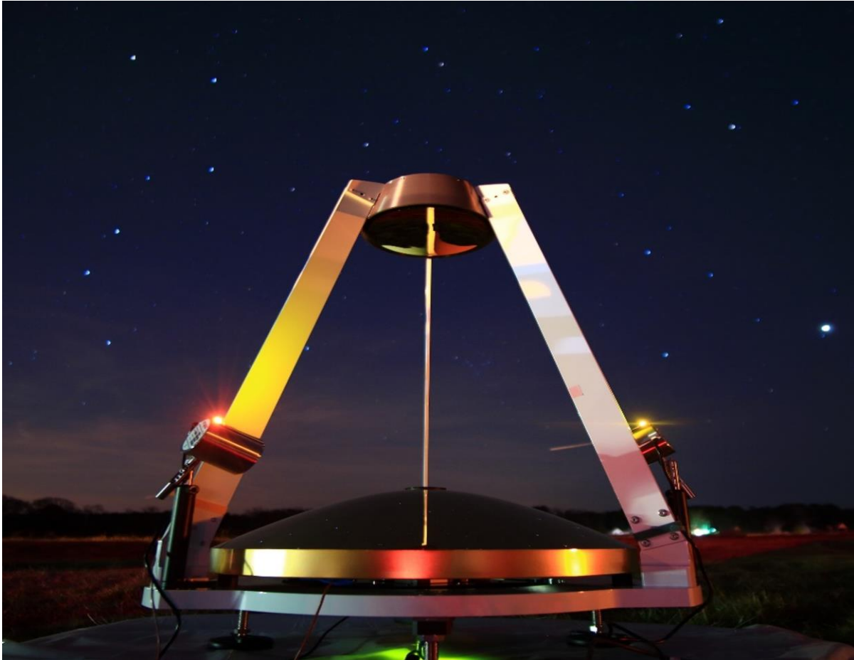
Fig. 1: MAMBA undergoing testing at night to measure atmospheric water vapor. Calibration black bodies are indicated by their power lights.
